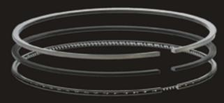
Now that engines are required to be more compact, lighter, and more sophisticated in performance, the choice of piston ring materials has been widened to include steel in addition to the traditional cast iron. Moreover, in order to enhance their wear resistance and durability, they also undergo various surface treatments including nitriding and PVD treatment.
